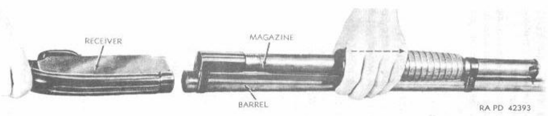
Figure 31—Barrel and Magazine Disengaged from Receiver—Winchester Shotgun M12 (Take-down)
